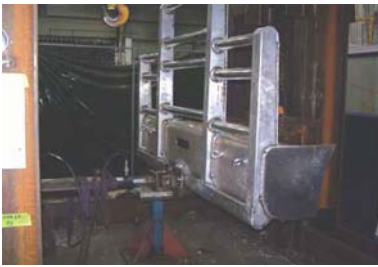
8 Tonne test @ P3 test point
