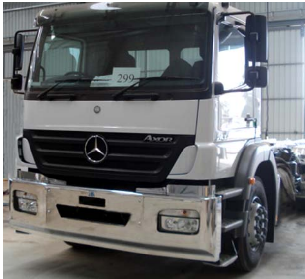
ADV7705 MERC AXOR "Texas" FUPD Bumper only suitable for trucks without factory FUPS Approval No. FUP10127/09
