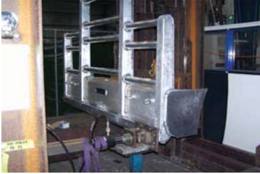
8 Tonne test @ P1 test point
